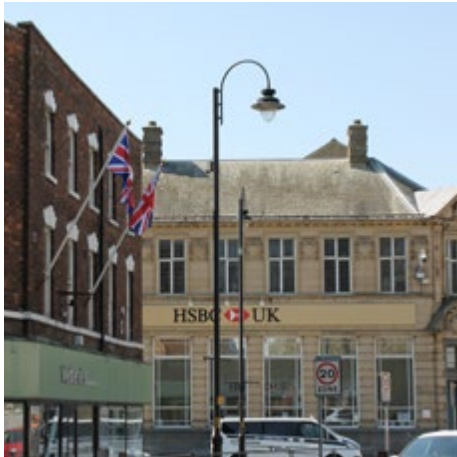
6.25 Curved luminaire style suited to more modern contexts on A19
