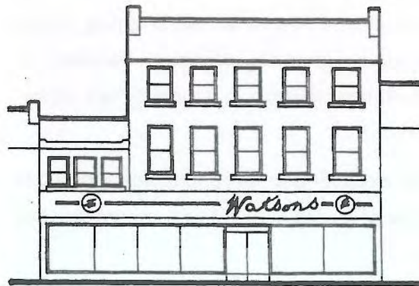
Shop front which does not respect the building above
