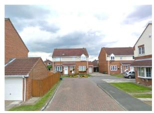
5.15 The plots are equally sized and are either open-plan or have a low brick wall. Shrubs and bushes mark boundaries and soften the built form. The houses are a standard square design and are detailed with a smooth cream render at first floor, and canopies and porches on the front door. Most houses have bow windows at ground floor, and there are occasional gable roof over first floor windows introduces a detail to complement the dentil course at the eaves.
