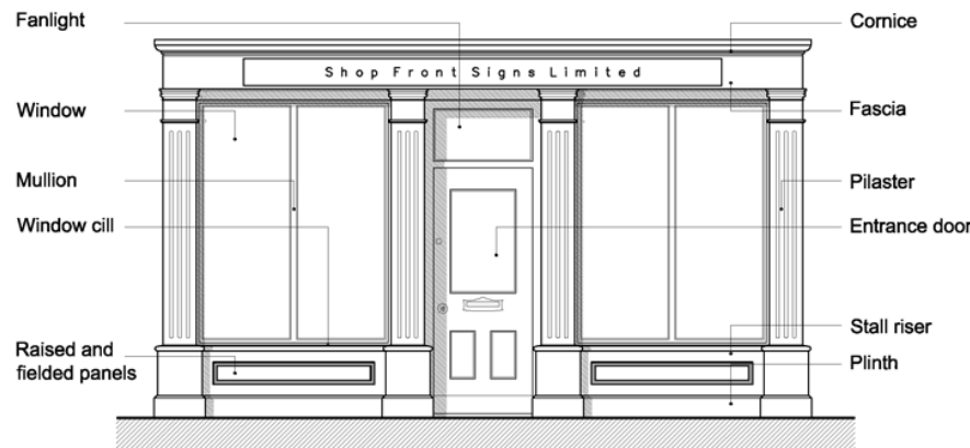
Figure 9: Typical late Victorian style shopfront.
