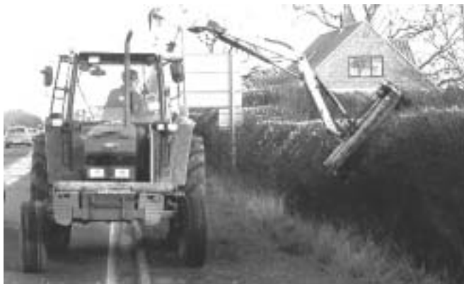
A Reciprocating bar cutter in action.
