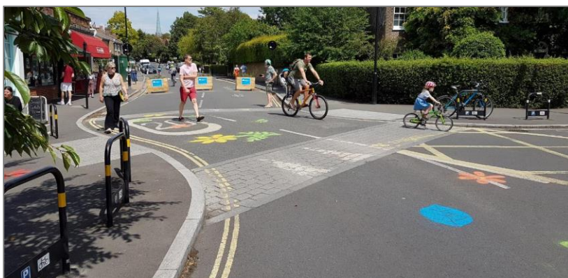
Figure 3.12. Modal filter / LTN
