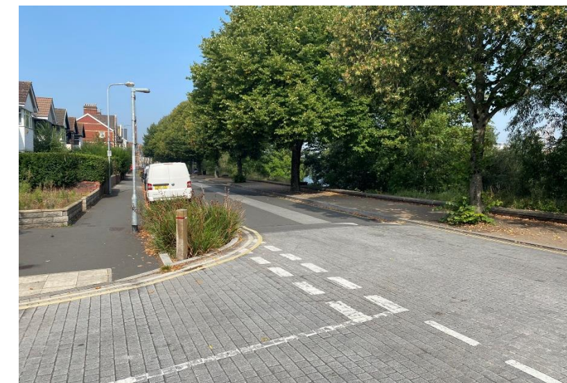
Figure 4.5. Buildouts with SUDs
