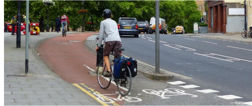
Figure 3.7. Segregated cycleway (carriageway height)
