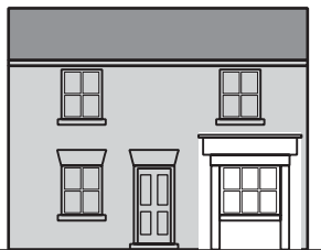
Pilasters continued down to the ground.
