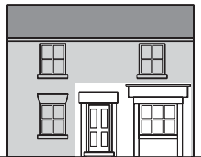
Door given a surround to match the window (door & window are still separate elements).
