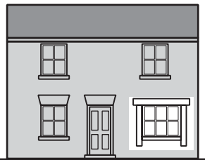
Enlarged window, with emphasised surround.
