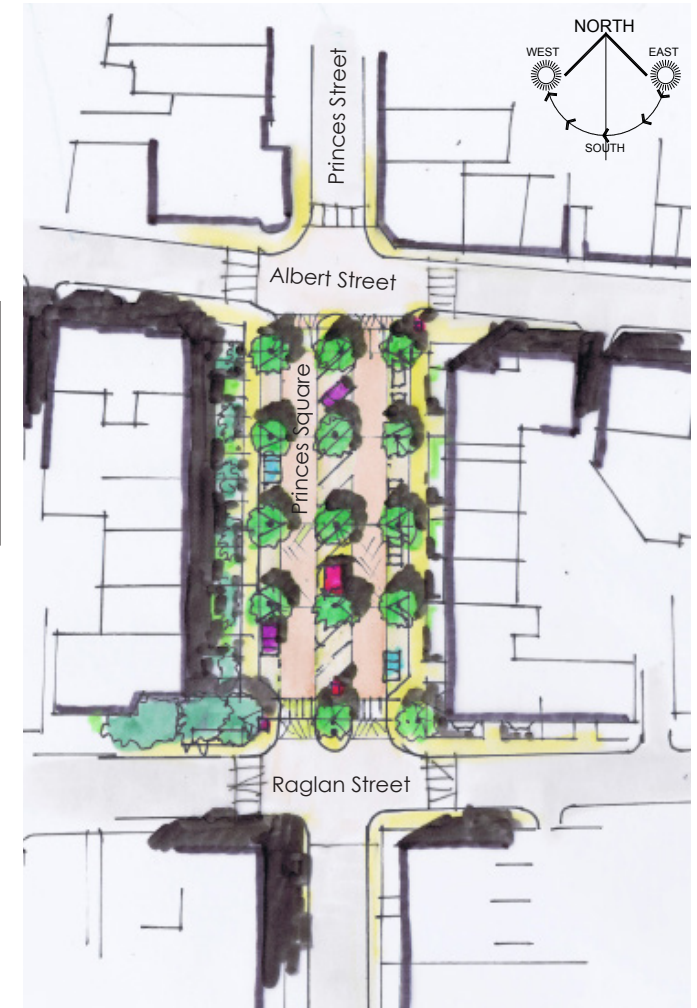
Above: Indicative layout of the new Princes Square with reduced on-street car parking, dedicated "cycle hub" and new planting.
