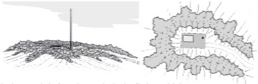
Fig.6. Mounding to conceal cabin, fence and access track and seeding of local grass and shrubs on open ground, e.g. moorland, heathland.
